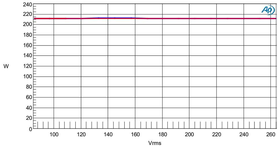
Figure 11: Output power vs. mains, mains freq. 50 Hz (blue), 60 Hz (red)
