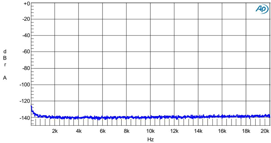
Figure 7: Idle noise spectrum, 0 – 20 kHz @ 0dB = 200 W / 4 Ω
