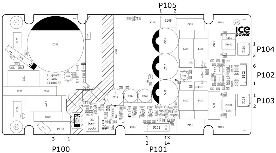
Figure 2: ICEpower200AS2 connector overview
